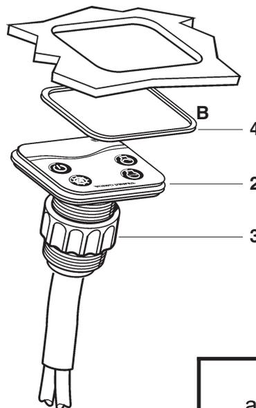
Avoid installing the cable with a sharp bending radius at the connector, to retain its sealing function.
